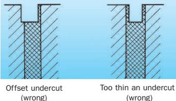
Commutators with flush mica against the copper segments require very hard brush material with the consequence of high commutator wear. For a better lifetime, it is necessary to undercut the insulation (see sketches).
