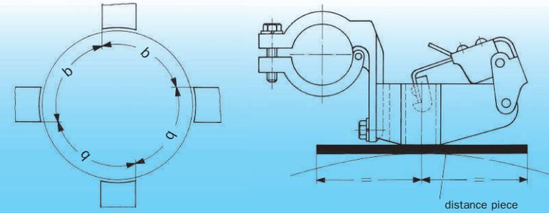
The distance between the commutator and the lower edge of the brush box should be set at between 1.5 and 2.0 mm. If the commutator has been remachined, the brush holders will have to be reset to maintain this distance. The setting of the brush holders should be done with a distance piece.
