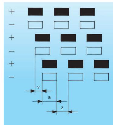
The fitting of brushes on the commutator must be carried out either exactly radial or at a certain angle, which is then called either a trailing or a reaction position, according to the direction in which the commutator rotates. The trailing and reaction position are used in order to reduce vibrations.
